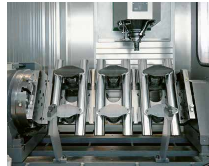
Complex hydraulic clamping unit, modularly designed by AXA, for quick conversion and secure chip flow
