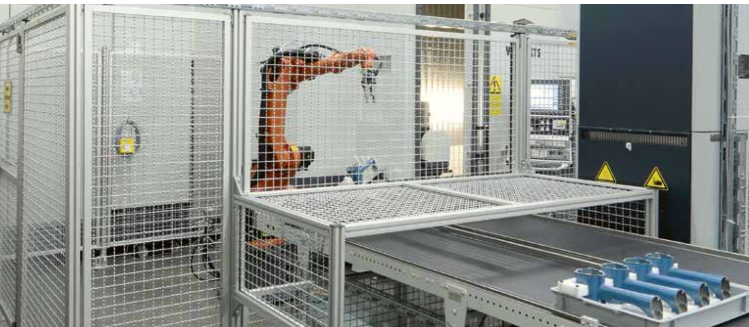
Machine buffer store reduces set-up times due to long transport distances of the robot system - During machining, the robot changes the workpieces from the buffer into the workpiece storage unit
