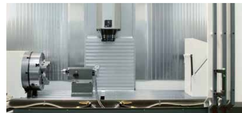
Rotary table combined with a tailstock as well an additional pick-up station for special tools, angular heads or multiple spindle heads
