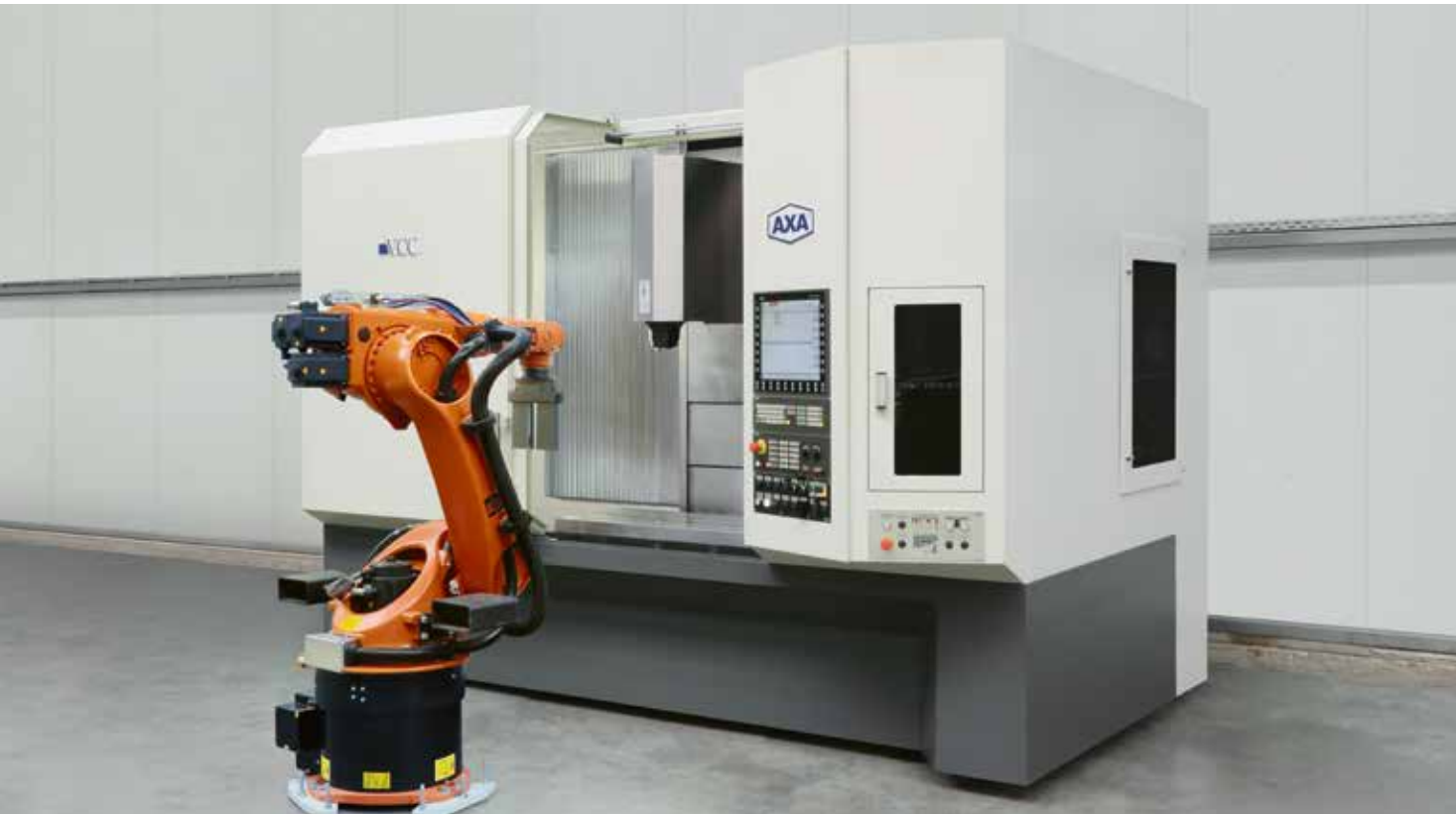
Installed industrial robot in front of the travelling column machine for direct machine loading and unloading with workpieces
