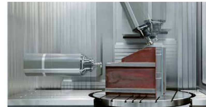
The tilting spindle head in operation: enables the machine to work in a range of \pm 100^\circ
