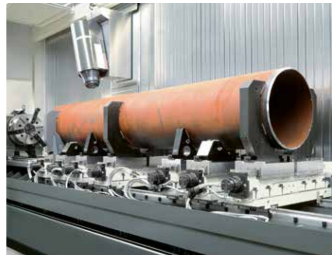
Manual or NC-driven pre-centering and presetting of the clamping elements for the next workpiece diameter
