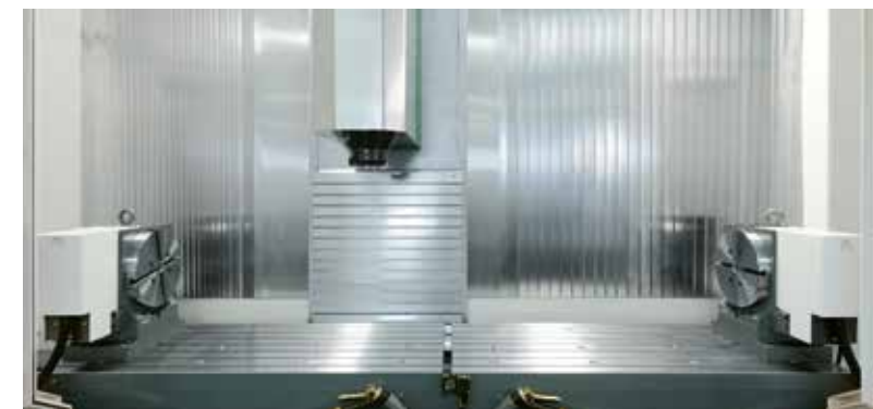
Rotary table in the left and right workspace or rotary tables in gantry mode for clamping bridges in long bed machining mode
