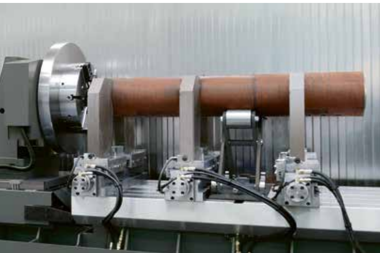
The workpiece can be rotated to position when clamped
