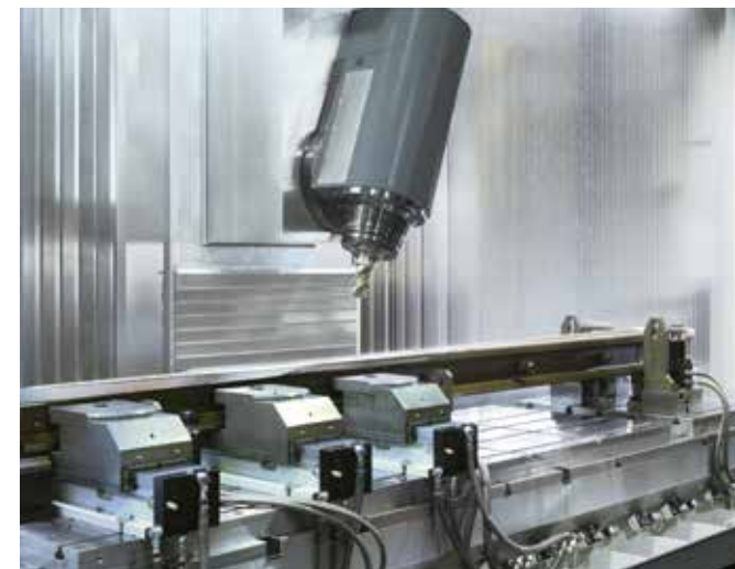
In the right hand working space long strips can be manufactured in clamps that can be positioned flexibly
