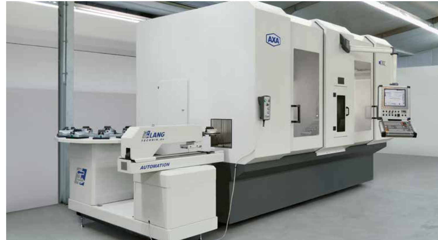
Quick and simple automisation by compact complete solution with workpiece storage, handling system and zero-point clamping
