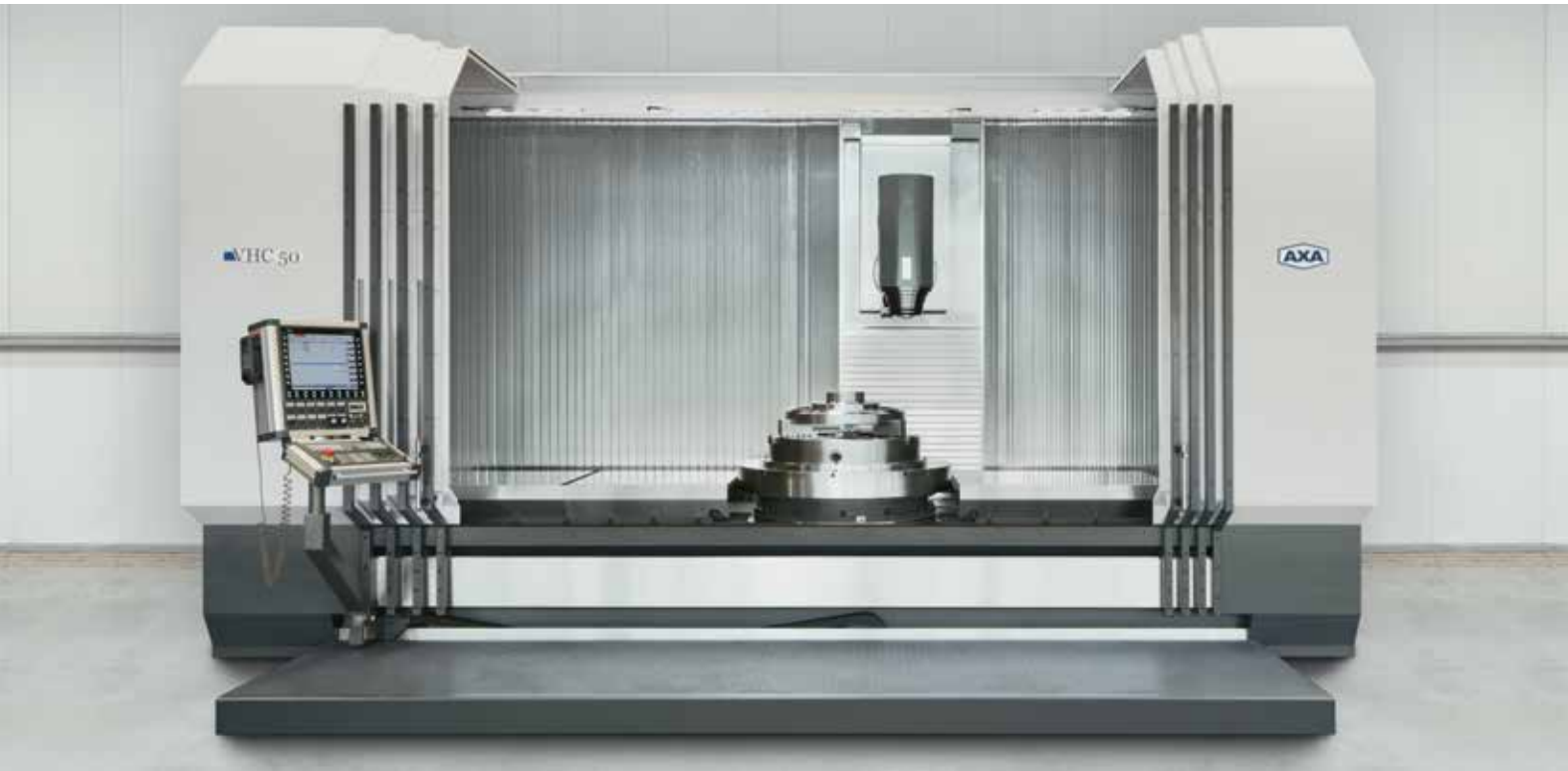
Milling, drilling and turning in one setting with vertical and horizontal spindle position
