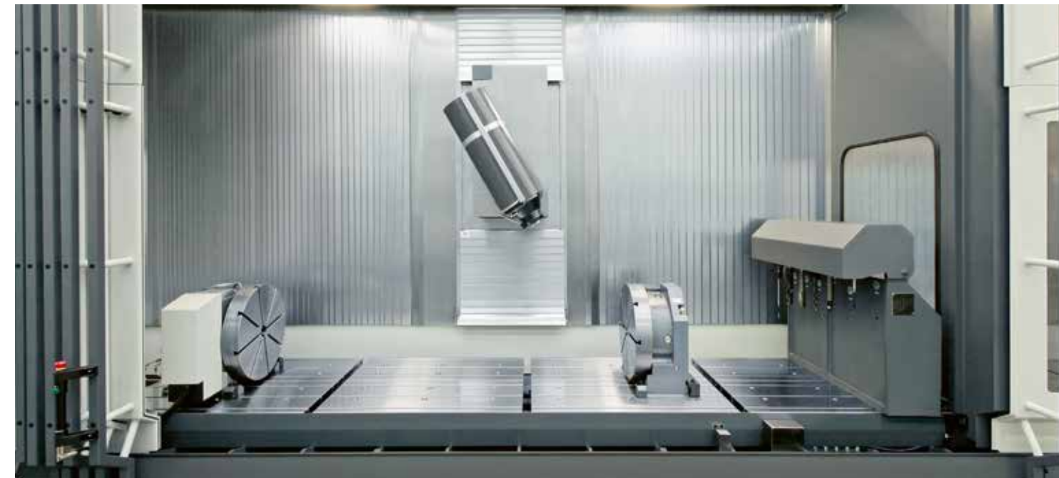
Rotary tables in gantry mode for clamping bridges as well as further, removable pick-up station left for pendulum operation or right for long bed operation
