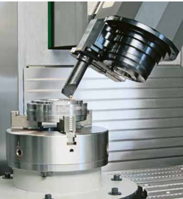
All intermediary angles can be set on the turning tool position beside the vertical and horizontal spindle position
