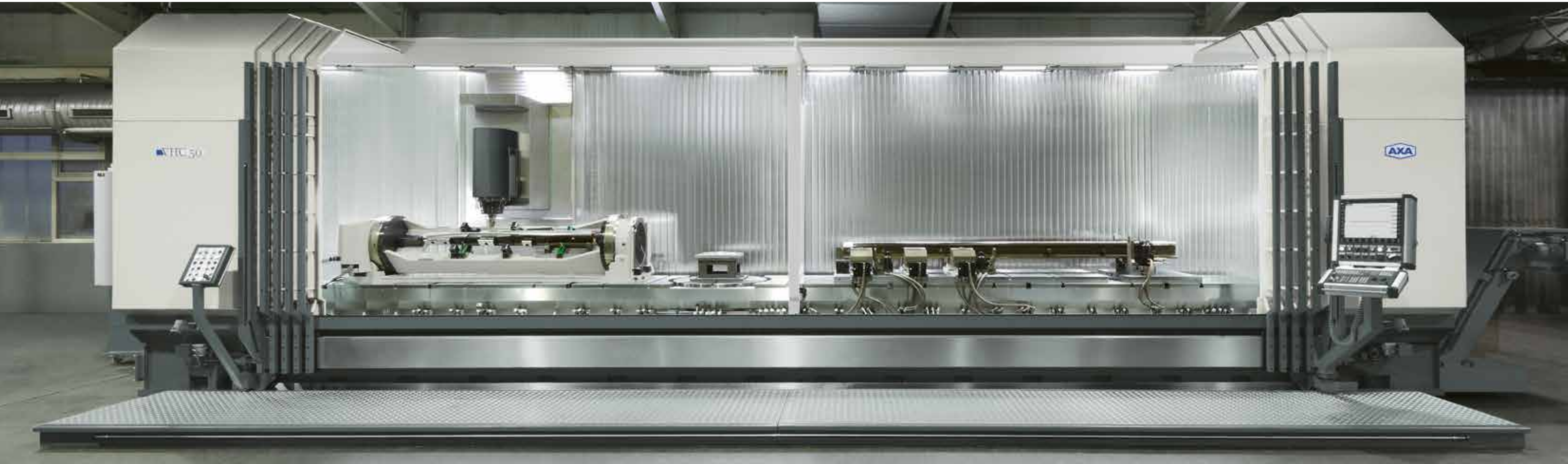
The heavy SK 50 pendulum machining centre is fitted with a high-performance tilting spindle head - Different clamping devices allow different workpieces to be machined in parallel
