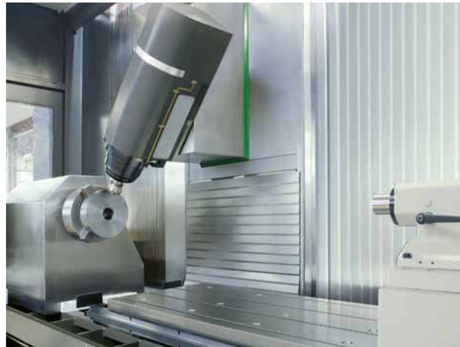
Turning spindle with 1500 rpm in combination with a tailstock that can be manually adjusted over the fixed machine table in longitudinal direction for varying lengths of the turning workpieces
