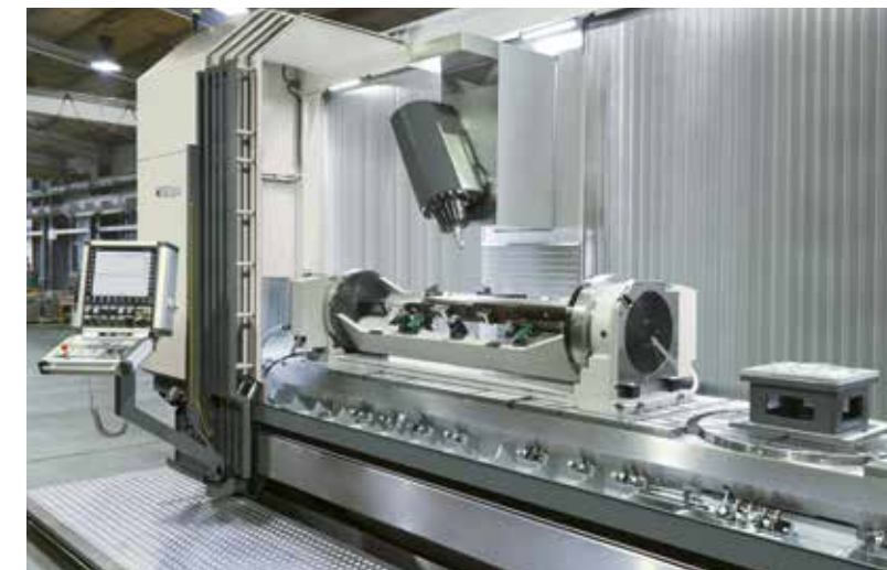
Two NC rotary tables working in gantry mode ensure torsionally stiff suspension of the long clamping bridge in the left-hand pendulum working space
