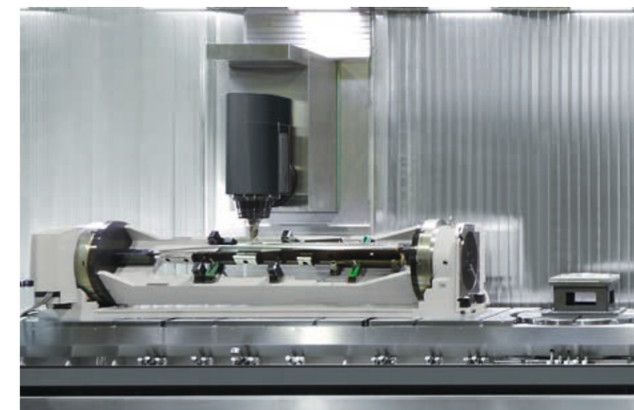
Two NC rotary tables working in synchronous operation ensure torsionally stiff suspension of the long clamping bridge
