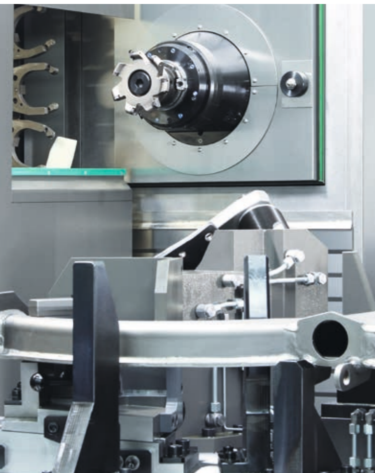
Tool change takes place behind working area cladding
