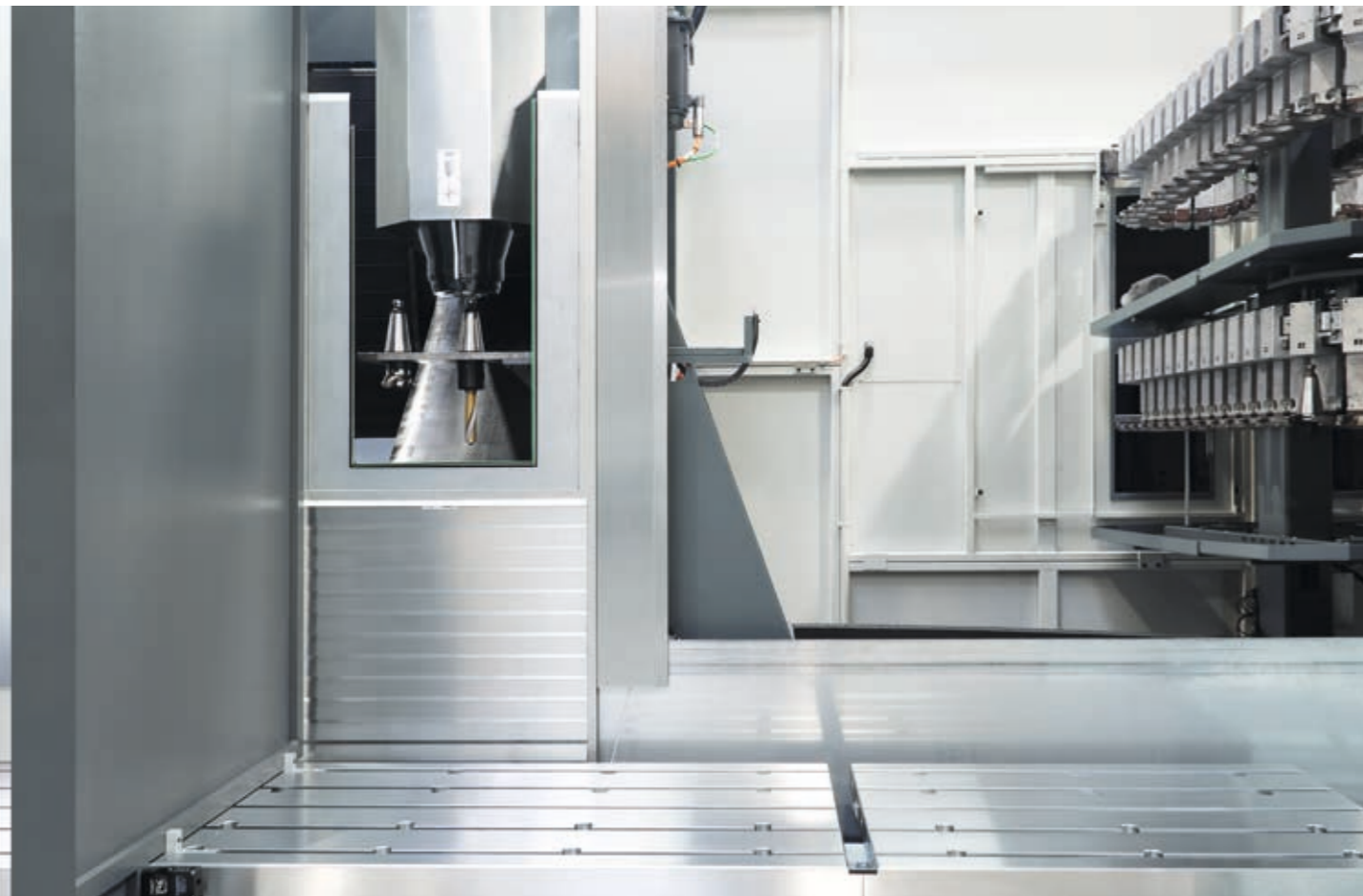
Tool change takes place behind working area cladding – The changer moves between the XTS tower and the spindle and makes the tool available by double gripping system
