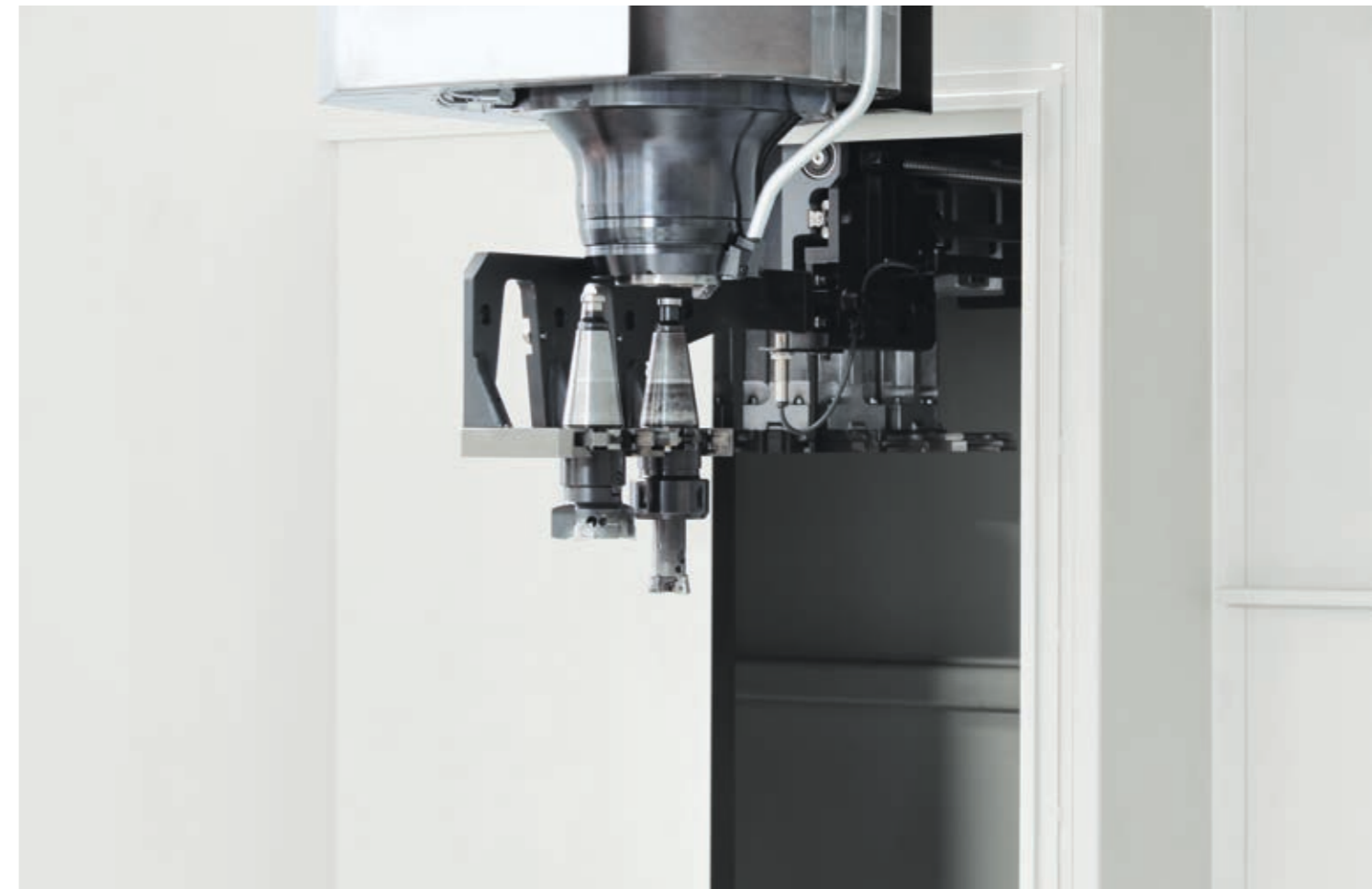
Tool pre-selection during machining and short tool change time by double gripping system
