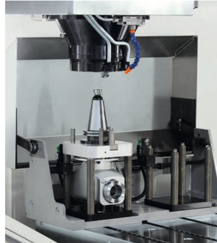
Vertical pick up magazine – Firmly integrated into the working area or optionally moved out of the working area
