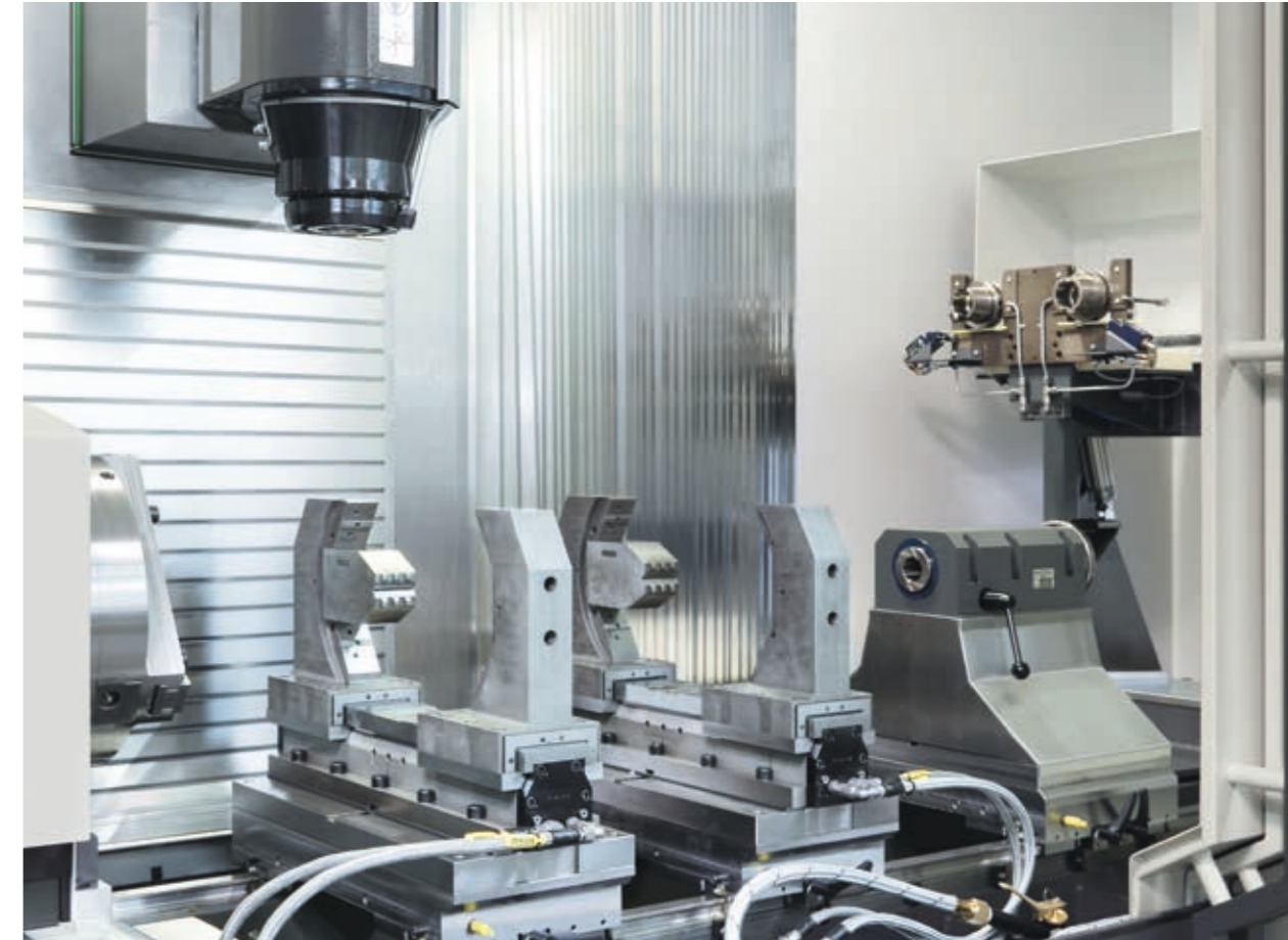
By the rotary table on the left and the tailstock on the right, the workpieces are automatically rotated into position for the centre clamping device
