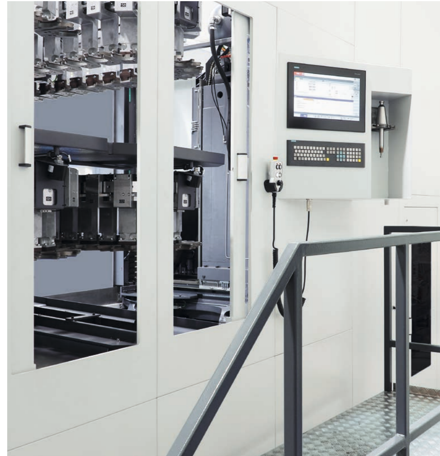
If there is more than one XTS tower then the tool magazine is loaded from the back rather than from the side
